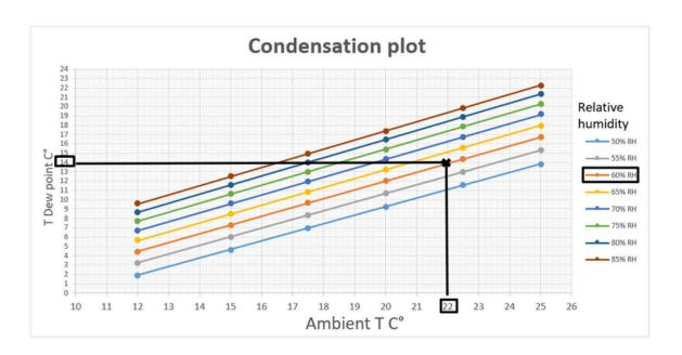
Knowing the ambient temperature, follow the '22 line' on the x-axis until it intersects with the 60% RH curve and you obtain the dew point on the y-axis. Dew Point =  $14^{\circ}C$  (57°F)
