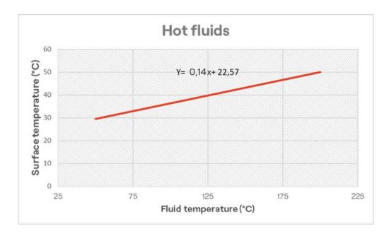
TELCRA<sup>®</sup> performs at high temperatures, providing good insulation and ensuring surface temperatures suitable for skin contact, to help prevent burns.
