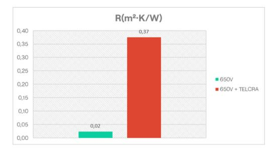
The addition of TELCRA<sup>®</sup> insulation improves the thermal resistance of the resulting construction from 0,02 to 0,37 m<sup>2</sup>·K/W.
